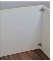
The range hood will act as a vent. Lay it on top of Side E (top piece) and mark where the attachment holes are. Remove the vent and drill a hole in the middle of each circle with your 3/8-inch drill bit.Lay side E and Side B with corners end to end. Side E goes on top of side B's top edge. Apply a thin layer of Gorilla Glue according to instructions. Press ends together and secure with L brackets. It really helps to have an extra pair of hands to hold
